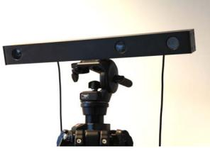
Figure 2. Our customized trinocular stereo camera setup with a baseline of 40cm (between the left and right cameras).
