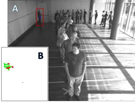
Figure 4. Loitering detection. A) An individual is behaving with a suspicious path and spending a significant amount of time off the queue. B) The associated trajectory, which led to the abnormal detection. Dots in the trajectory represent stop or change direction points.
