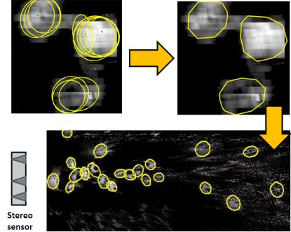
Figure 3. Top-left: Stable clusters estimated for a fast scale-adaptive CamShift method. Top-right: Computed convex hulls delineating the final objects. Bottom: Sample detection results in a queue seen from the top.
