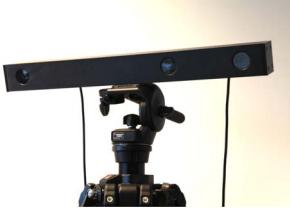
Figure 2. Our customized trinocular stereo camera setup with a baseline of 40cm (between the left and right cameras).
