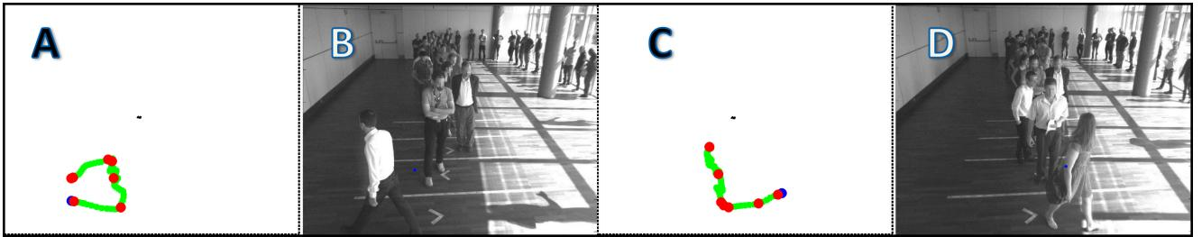
Figure 5. Wrong path detection. A) Mobile trajectory detected as abnormal. B) Individual undertaking wrong queue exit. C) Mobile trajectory detected as normal. D) Individual undertaking normal queue exit.
