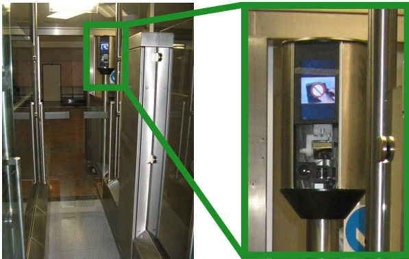
Figure 1. eGate from the inside with a detail view of the face camera
