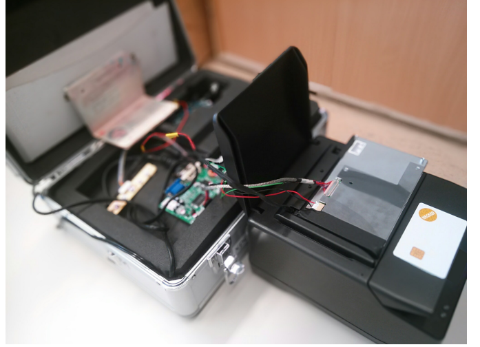
Figure 2. The proposed document simulation setup running on a dedicated hardware. The display simulating a passport as well as the brightness sensor (red and black wires) are placed together on the document window of a reader device. The simulator is controlled via wireless network from a nearby laptop.
