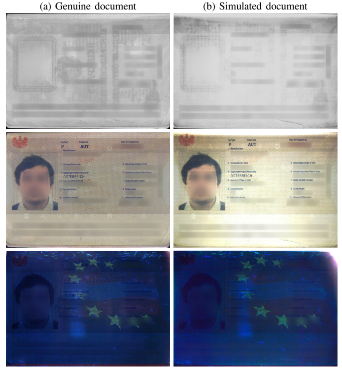
Figure 4. Side-by-side comparison of images obtained by a document reader for (a) an Austrian ePassport and (b) a simulated version of the same document. Rows comprise images associated with different spectral channels, i.e., IR, White, and UV, respectively. Images of the genuine document were used as templates in the simulation.
