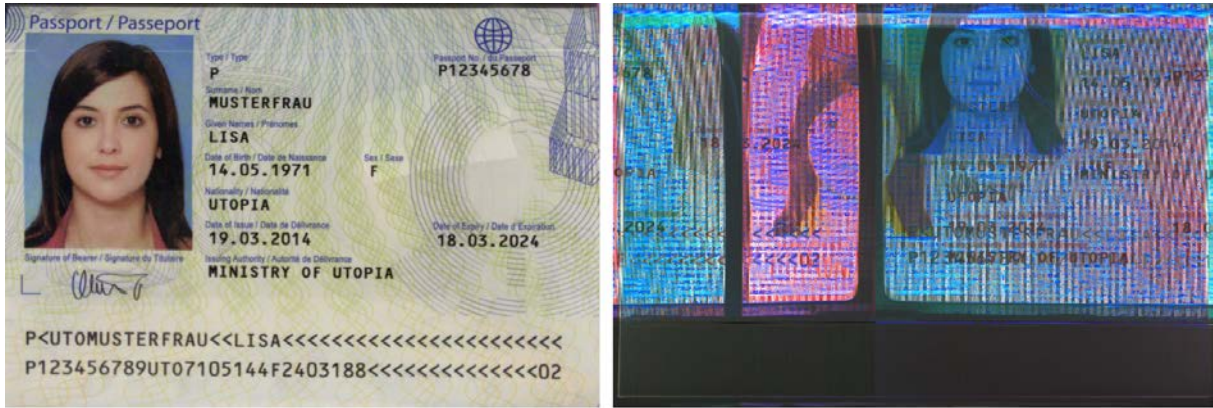
Figure 3 Comparison of a correct readout (left) and a failed readout (right) during HPEM exposure
