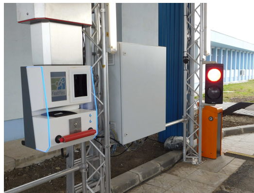
Overview of the FastPass installation at the land border crossing point in Moravita (Romania): kiosk for enrolment in the booth (left side); device for document scanning and face capture (on the right side) . © FastPass consortium
